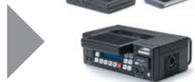
Remove the Storage Module or ExpressCard 34 media from Ki Pro.
