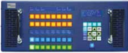
▲ Front panel With the Spyder X20, layers can be in 'program' and in 'preview' mode. You can build preset displays in preview mode using live layers without affecting the display being viewed by the audience.
