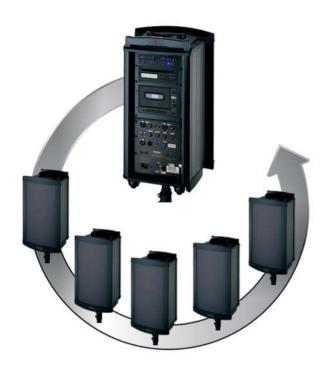
Audio Link allows the inter-connection of the RoadMan 102 unit with up to 20 SLAVE units to from a large network of amplified speakers. In order to do this, the MASTER unit with the audio sources (wireless mic, wired mic, cassette or CD) is connected to the SLAVE unit via the ACTIVE OUT connector. The ACTIVE OUT of the SLAVE is then connected to the ACTIVE IN of the next SLAVE and so on if more SLAVE units are required.
